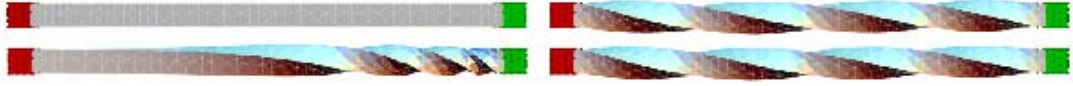
Figure 7.2: Behavior of our deformation technique when a 360^\circ twist is applied to the green handle. Top left: Original model of a bar; Bottom left: result after applying the twist without rotation interpolation; Top right: deformation without rotation interpolation converged after several seconds; Bottom right: instantaneous result with rotation interpolation.
