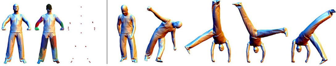
Figure 9.1: Animation of a scanned character using optical MoCap data. From left to right: Input model, reduced tetrahedral model with rigid regions marked roughly, 22 input handles, five frames out of a cartwheel sequence.
