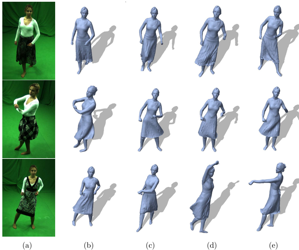
Figure 10.6: Results for skirts 2, 3, and the dress model (from top to bottom). Column (a) input frame from reference sequence; (b) the reconstructed animatable model simulating the same pose; (c)-(e) subsequent frames of a newly created animation for which only motion parameters of the underlying skeleton were given.
