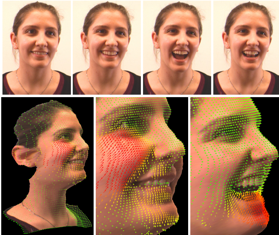
Fig. 3. Results for real world sequences (image size 470 \times 340 ). Top Row: (a) + (b) Smiling , left frames at consecutive time steps. (c) + (d) Closing Mouth , left frames at consecutive time steps. Bottom Row: (e) Reconstruction and overlaid scene flow for Smiling . Increasing magnitude from green to red. (f) Close-up Smiling . (g) Close-up Closing Mouth . Runtime: \sim 260 seconds. Parameters: \alpha_1 = 15 , \alpha_2 = 20 , \alpha_3 = 15 , \beta_1 = \beta_2 = 0.5 , \gamma = 30 , \mu = 1 .
