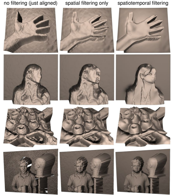
Figure 8: Mesh renderings of distance maps without filtering, with spatial and spatiotemporal filtering. The last row shows data captured using a Microsoft Kinect sensor, with holes and depth quantisation steps. It is essential to refer to our video to see the full improvement of our approach.
