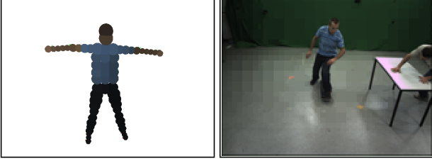
Figure 2. SoG model overview. Left : Body model generated from example input images. Right : Image SoG approximation generated from a quad-tree (each cell represents one Gaussian).
