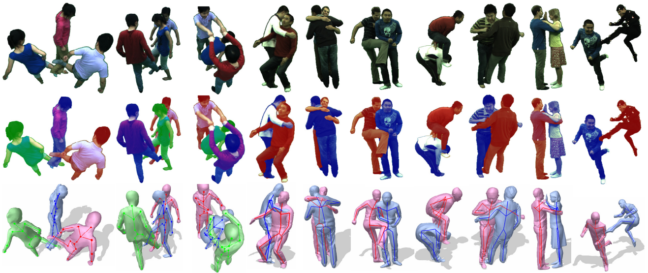
Fig. 11. Markerless motion capture results. First row: input images after background subtraction; second row: their corresponding segmentation results; third row: estimated surfaces and skeletons. From left to right: Hop , Crossover , Bend , Wrestle , Hug , Hit , Jump , Crash , Couple-dance , and Fight .
