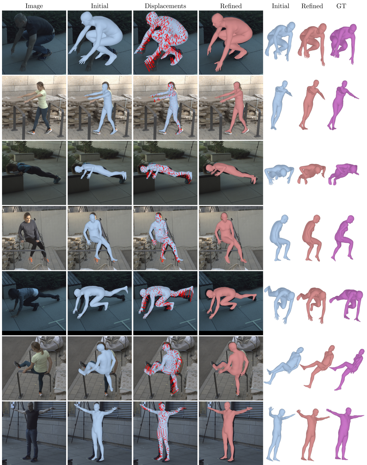
Figure 2. Additional results from the RICH [9] dataset. From left to right: input images, initial body estimates, our predicted displacement fields, our refined 3D human models and side views of initial, refined and ground-truth bodies.
