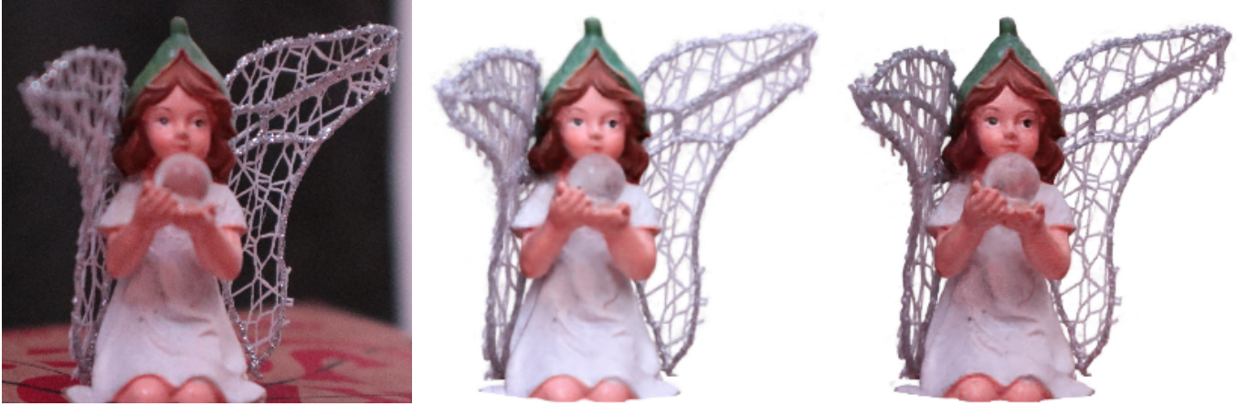
Fig. 1. Left: a 5\text{cm} \times 8\text{cm} \times 6\text{cm} figurine captured with an f/5.6 aperture, ( center ) reconstructed with instant NGP [Müller et al. 2022], and the proposed f NeRF ( right ). The reference image on the left was not used for reconstruction. While previous methods bake the defocus blur in to the radiance field, our method does not and reconstructs sharp details at all depths. It achieves this by successfully aggregating the radiance information from views close to the focus plane while simultaneously combining radiance values further away from the focus plane using a physically meaningful defocus model.
